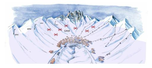
GINA® records the ground vibrations caused by avalanches and enables the detection of both natural and preventive avalanches (see figure below).
