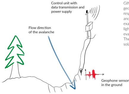
GINA<sup>®</sup> consists of a control unit and a geophone sensor. The control unit is responsible for data transmission via mobile radio and for communication with other devices, for example with any connected avalanche traffic lights, while the sensor continuously records and evaluates ground vibrations.
