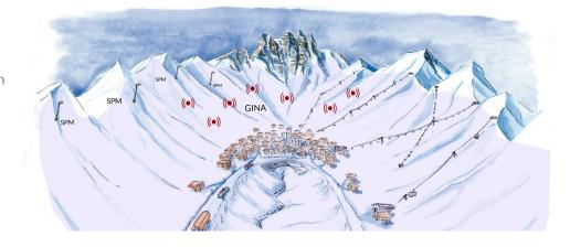
GINA<sup>®</sup> records the ground vibrations caused by avalanches and enables the detection of both natural and preventive avalanches (see figure below).
